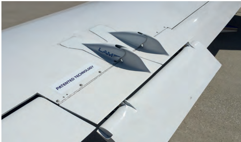
Above: The LAM Aero System is the first major new wing flight control system since the introduction of the aileron and flap
